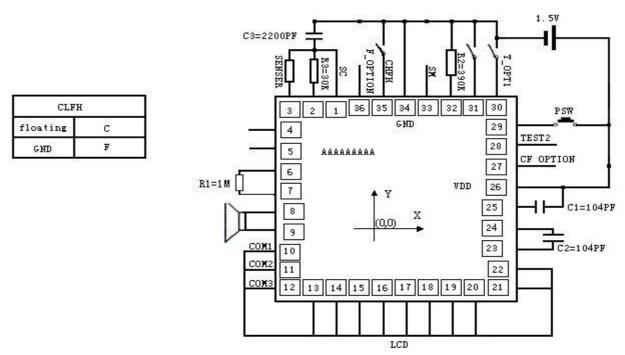
Note: The value of R1, R2, C1 C2 is allowed the tolerance of  $\pm 5\%$ .
