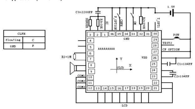
Note: The value of R1, R2, C1 C2 is allowed the tolerance of ±5%.
